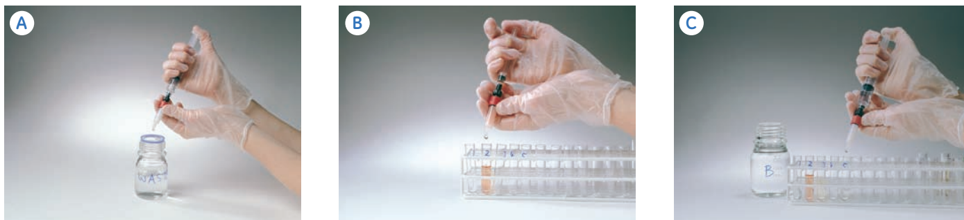
Fig 10. Using HisTrap HP 1 ml with a syringe. A) Prepare buffers and sample. Remove the column's top cap and snap-off the end. Wash and equilibrate. B) Load the sample and begin collecting fractions. C) Wash and elute, continue collecting fractions.
