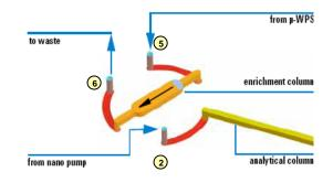
Port 5 of the HPLC-Chip Cube micro valve is connected to the  $\mu$ -well-plate sampler. The loading solvent is directed to waste through Chip cube micro valve port 6. Chip Cube micro valve Port 2 is connected to the nano-pump
