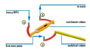
Port 6 of the HPLC-Chip Cube micro valve is connected to the  $\mu$ -well-plate sampler. The loading solvent is directed to waste through Chip Cube micro valve port 5. Chip Cube micro valve Port 2 is connected to the nano-pump.
